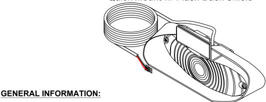
Flash tube rated 25 watts. Compact individual unit  $2\frac{1}{4} \times 6\frac{1}{2}$  inches. Equipped with an 8 foot cable for easy routing and can mount anywhere. Available with grill, window or bumper mount brackets. Choice of RED, BLUE, AMBER, or CLEAR polycarbonate lenses. Requires remote power supply.
